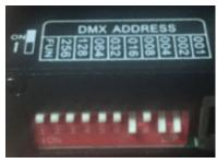
DMX initial address = 1+2+8, the initial address is 11, the corresponding addresses for conversion are 11, 12... (DALI device number + initial address-1).
