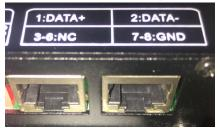
DMX signal port interface, two network port terminals are connected in parallel, port 1 is DATA+, port 2 is DATA-, port 3-6 is empty, port 7, 8 is GND.
